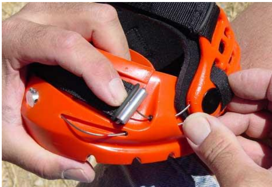
11. There are two methods for moving the cables. One method is to push an outward bulging loop in the cable like this.
